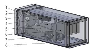
Fig. 1. Ozone generator structure: 1 – fan guard; 2 – Foxconn PV123812DSPF fan; 3 – frame;
