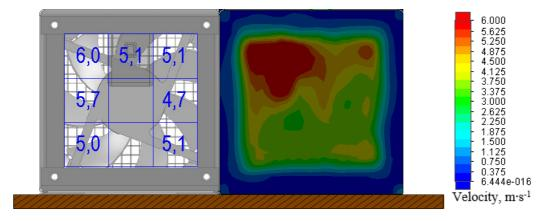
Fig. 6. Comparison of experimental measurement and simulation of air flow velocity
