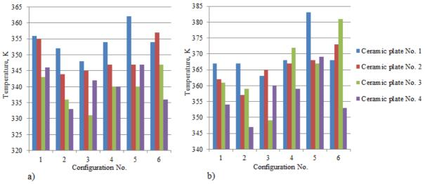
Fig. 3. Temperature of corona discharge plates for different configurations: a – average temperature; b – maximum temperature
